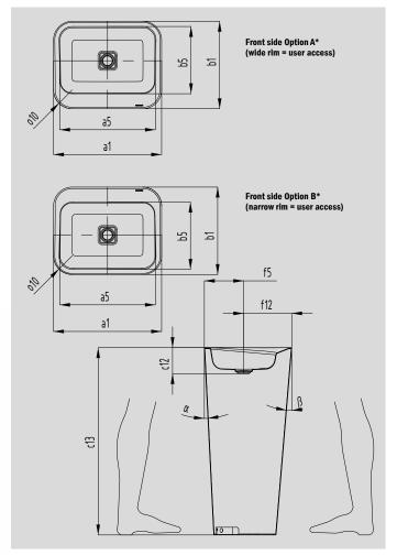
Pure freedom – the centrally-placed waste allows a choice of washbasin positions for installation. Choose your preferred front side from the above installation options.
